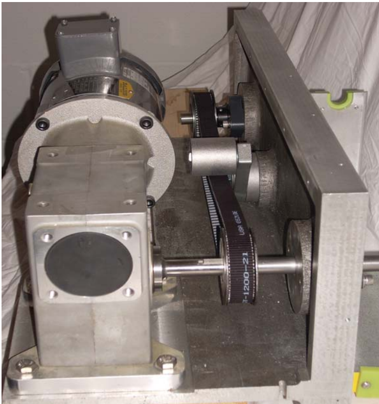
Rear Drive System (shown with rear safety cover removed)
